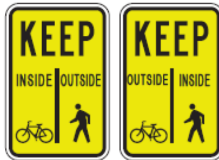
Figure 13 Recommended Bridge Bicycle/Pedestrian Signage
