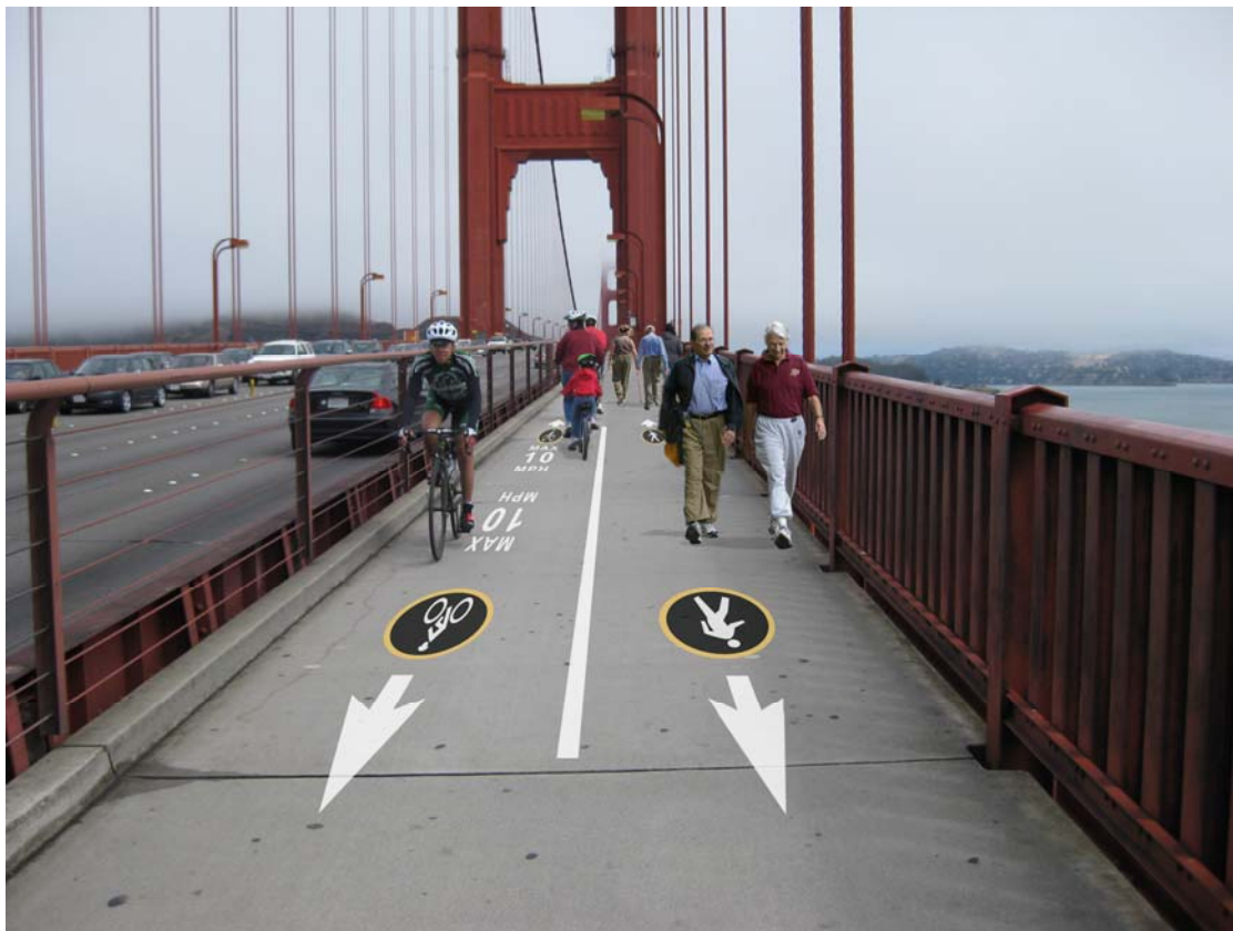
Figure 15 Recommended Pavement Markings
